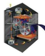
Through-Air Drum Drier Features Diagonally Offset Drums to increase Drying Area.
